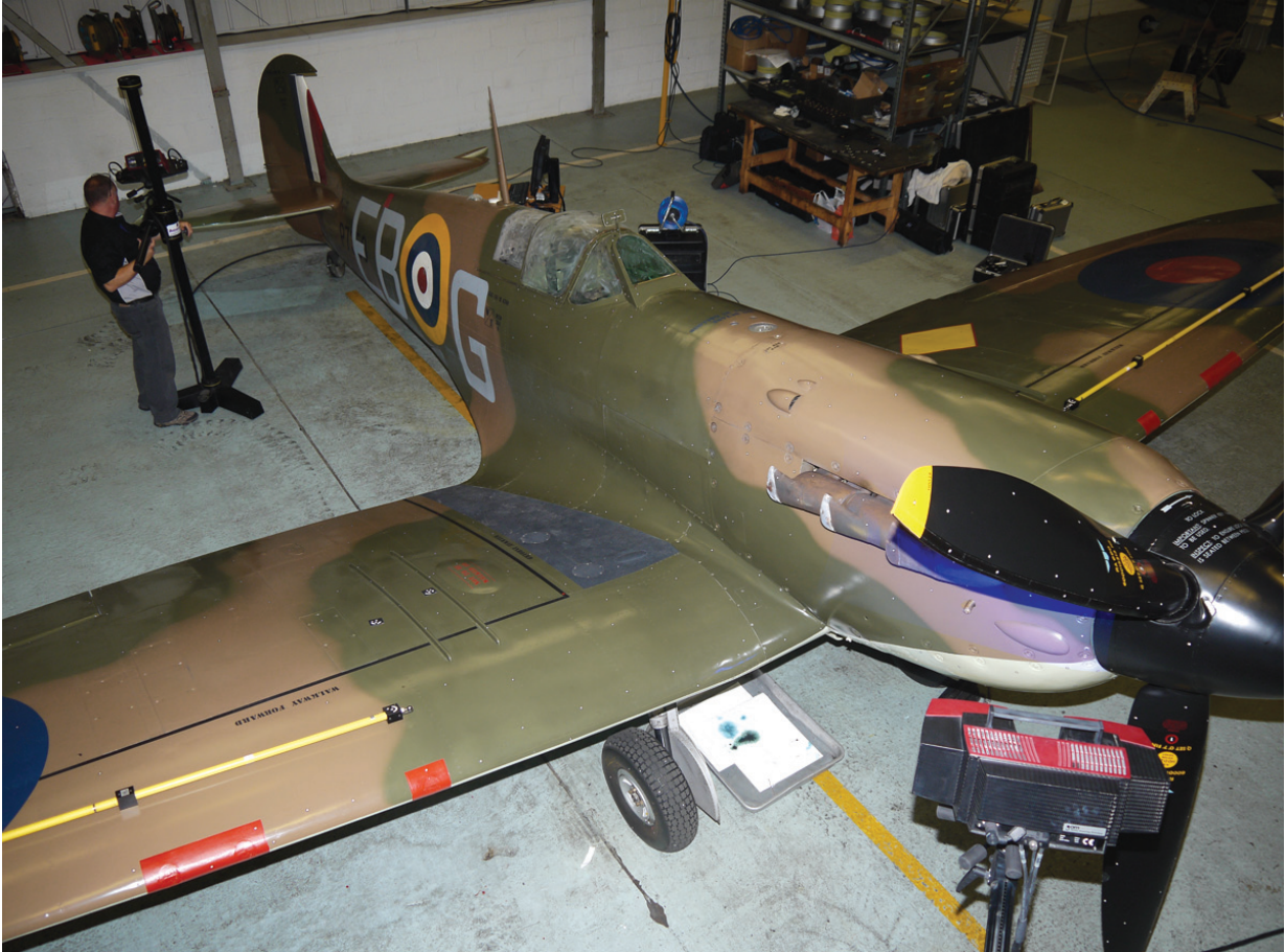
Shop personnel are scanning the last remaining WWII Spitfire that saw active service in the battle of Britain, for historical reasons and reverse engineering.
