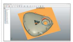
• It's a pretty quick process to build up the primitives you need to build off of this part, but one area that would prove tricky is manufacturing a gasket as there are no clear primitives available.
