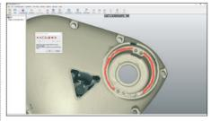
Now you can start to select your mesh faces to build your geometry from or to perform an alignment proceedure. The selection tools range from simple painting with the cursor to curvature-based flood filling.
