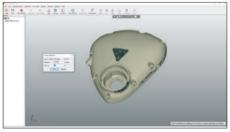
② The next step is to create a more efficient mesh to work off. QuickSurface doesn't need the heavy datset from the scanner, so includes a polygon reduction tool. This dataset was reduced by 20% from half a gigabyte.
