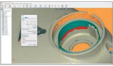
• The Cylinder primitive tool will a particularly useful tool for those looking to reverse engineering for building additional parts off. You have control over position, finetuning and the ability to make concentric with others.
