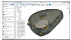
• The data from your work in QuickSurface can then be read in your workhorse CAD system. Here, we have the mesh-data alongside the extracted surfaces, used to redesign a part to match the physical part's form.
